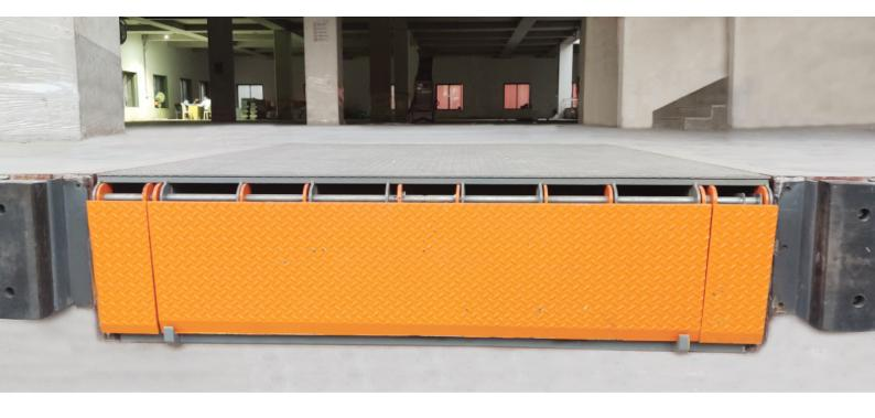
The Dock Levelers are a bridge that match the warehouse edge with Vehicle height. Its hydraulic system adjust the platform and the swinging hinged lip, which eventually rests on vehicle bed acting as a bridge between the loading area and vehicle to enable a safer movement for forklift to handle the material on or off the vehicle.
